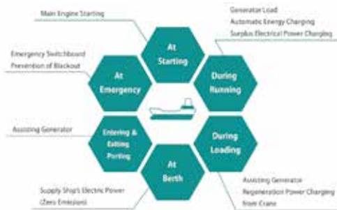
Fig.1 Applications of Li-ion Batteries on Ships
