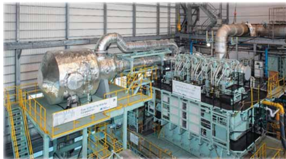
Shop test of 6S46ME-B8.5-HPSCR engine
