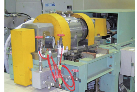
Test Equipment of 100mm shaft Dia. Result of Bench Test
