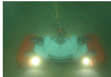
ROV undergoing cleaning work
