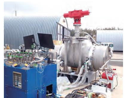
Prototype for LH 2 tests at JAXA Noshiro Rocket Testing Center (800A, 32" )
