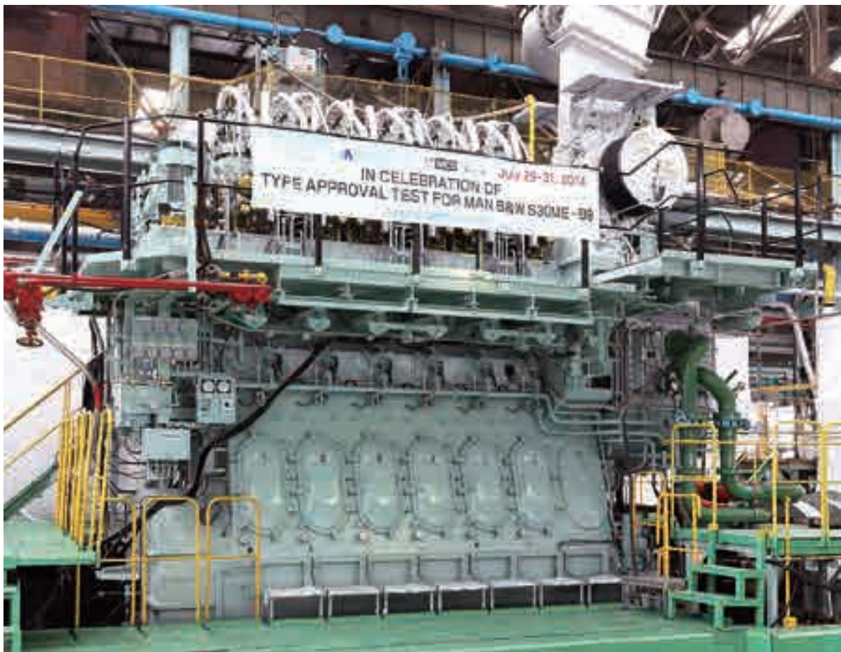
6S30ME-B9 Bore : 300mm / Stroke : 1328mm / Output : 3840kW x 195 min-1 / MEP :2.10MPa / IMO NOx regulation : Tier2 / SFOC : 176.0g/kW-h +5%margin at 100% load / Dry mass : 69ton
