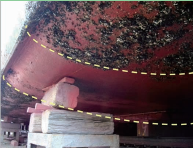
Barnacle free (1-year performance after long anchorage)
